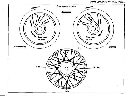
The key to correct lacing is the inside and outside spokes from the flange must slope down in the opposite direction as in the figure. The spokes are in opposite direction to the inner two spokes. In the group of four spokes laced, the inner spokes of each flange are sloping down in the opposite direction of the outer two spokes of the next grouping of four spokes and so on.
