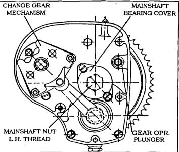
The gear box is bolied on to the back of the crankcase and has fourspeeds, which are foot-controlled, and a patented neutral finder. All gears are in constant mesh, changes being effected by robust dog clutches. The internal gear ratios are 2.77: 1 (1st Gear), 1.84: 1 (2nd gear) 1.36: 1 (3rd
