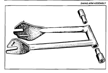
position of the spring box. The special tool for alignment of swing arm to be used. (PED 2044). No maintenance is necessary for the swinging arm pivot.
