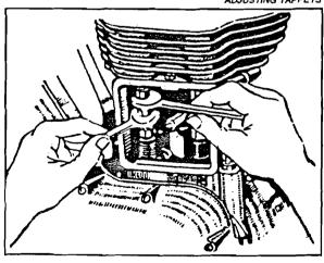
ADJUSTING TAPPETS amount of thermal expansion of the working
