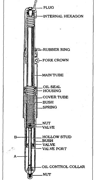
bump stroke and heavier on the rebound stroke, thus damping out any tendency to pitching or oscillation without interfering unduly with the free movement of the fork when the wheel encounters an obstacle or a pot hole.
