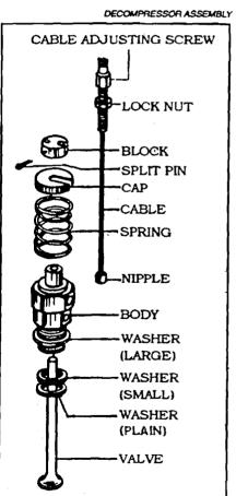
upwards and pull the cable nipple out of the body. It will now be possible to remove the cable and nipple through the spring, leaving the decompressor body and spring detached from the control cable.
