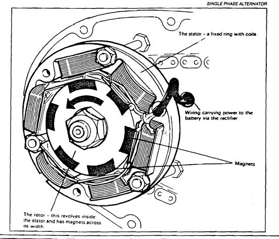
Fit the rotor first, making sure that it is located concentrically on the end of the drive shaft. Attention must be given to the proper seating of the key. Finally secure the rotor with the appropriate washer and nut.
